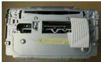
3.Remove the screws on the mental panel and take them apart
