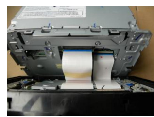
8.Fix the position of the cable so as not to interfere with the dish outlet, install the screen and lock the screws
