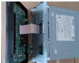
5.Remove the 60 PIN cable from the display panel(Be careful not to disassemble the socket of the display panel )
