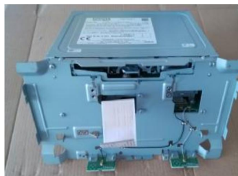
6.Use a screwdriver to remove the screws that fixed metal panel and remove the metal panel
