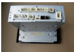
1.Remove the screws of the fixed display board
