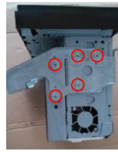
3.Use a screwdriver to remove the screws on the main assembly bracket on both sides of the head unit
