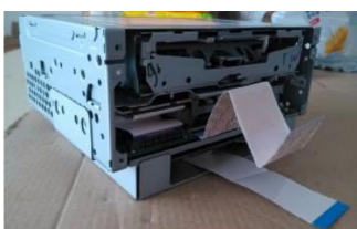
9.Put the navigation box to the bottom of the head unit as shown
