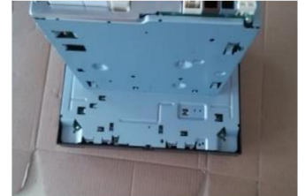
4.Use a screwdriver to remove the four screws on the back of the screen and remove the screen
