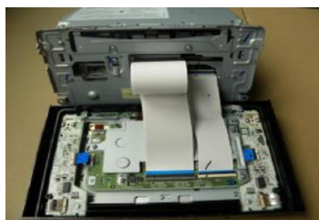
7.Insert the 80 PIN cable on the navigation box into the 80 PIN socket on the display board
