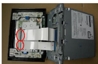
2.After the screen is disassembled, remove the cable that is connected to the screen
