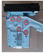
3.Use a screwdriver to remove the screws on the main assembly bracket on both sides of the head unit
