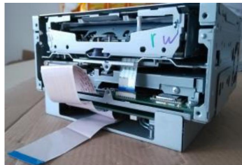
10.Insert the 60 PIN cable of the head unit into the sockets of the navigation box
