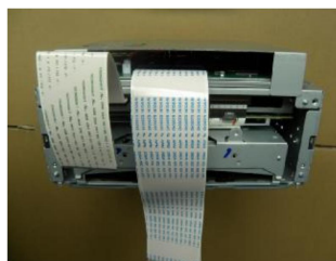
5.Put the navigation box at the bottom of the head unit, and then insert the 80 PIN cable into the 80 PIN socket of navigation box
