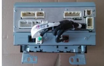
2.Pull out the cable behind the head unit
