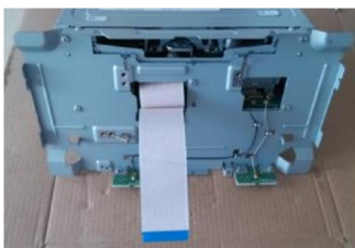
13.Insert the 60 PIN cable connected to the screen into the 60 PIN socket of the head unit
