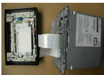
6.Put the cable from the metal panel outlet out,install the mental panel and lock the screw
