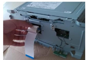
12.Put the cable from the metal panel outlet out, lock the screw, and then arrange the redundant part of cable and put inside the metal panel outlet
