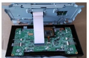
14.Insert the 60 PIN cable connected to the screen into the 60 PIN socket of the head unit. Finally install the head unit and lock the screws
