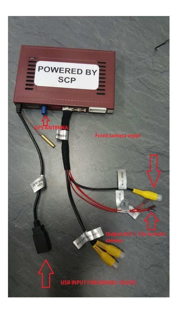
Connect the front camera to the included harness and connect the harness to the box as picture show.
