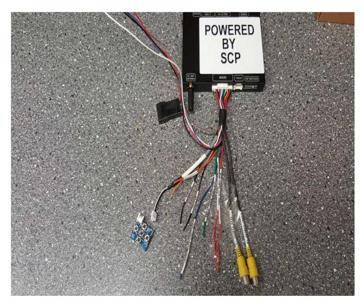
The system has 2 extra video inputs and they are marked front camera and rear camera.
