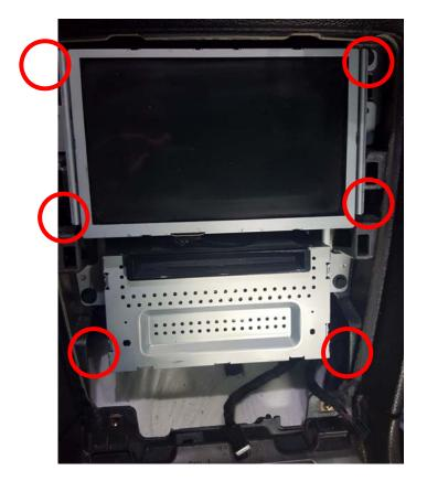
When the LCD panel is disconnected, you can open carefully ! : 5 screws (small Phillips screwdriver)
