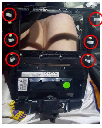
After You can remove the LCD Panel and the CD module: 6 screws (7 mm) - after disconnect the LCD panel
