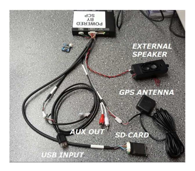
Install the Gps antenna in a good position under the dash and mount the external speaker behind the screen.
